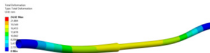
Fig.6. Deformation pattern of the gas pipeline with a sharp diameter transition from 700 mm to 500 mm within the landslide zone, with the pipeline ends fixed at the edges of the slope
