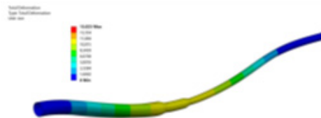
Fig. 14. Deformation pattern of the gas pipeline with a two-stage diameter transition from 700 mm through 500 mm to 350 mm (connected using two diffusers/cone reducers) within the landslide zone, with free lateral boundaries of the slope model
