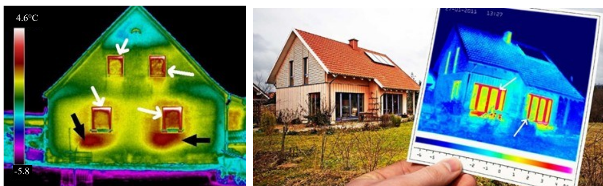
Fig. 1. Two examples of thermographic images of the facade of single-family houses: on the left an older building [3], on the right a newer building [4] The white arrows indicate the windows (frames) with highest surface temperatures [photos modified by the author].
