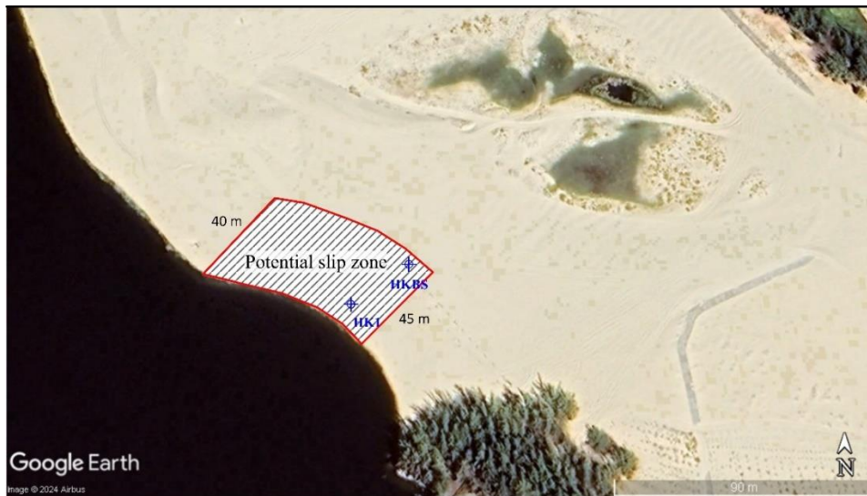
Fig. 6. Slip zone predicted from the geophysical results
