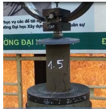
b) The sample at failure time
