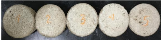
b) Samples are signed to prepare for doing the unconfined compression test
