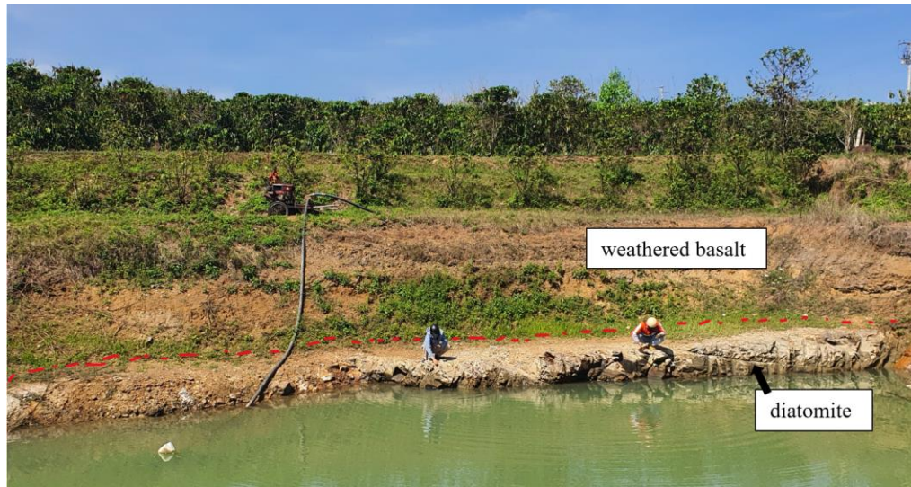
Fig. 7. Stratigraphic Relationship Between Diatomite and Basalt flows (weathered basalt) The diatomite is overlain by a layer of basalt (weathered basalt), with the boundary marked by a red dashed line.
