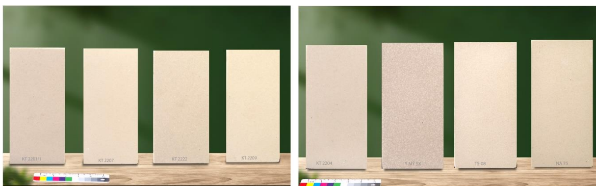
Fig. 16. The fired product samples consist of eight samples: five pegmatite samples, two Phu Tho samples, and one sample from the Y My factory, which is currently in production.
