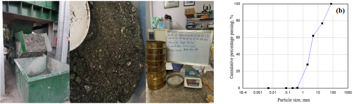
Fig. 2. a) Bottom ash from the Xuan Son plant; b) Particle size distribution curve
