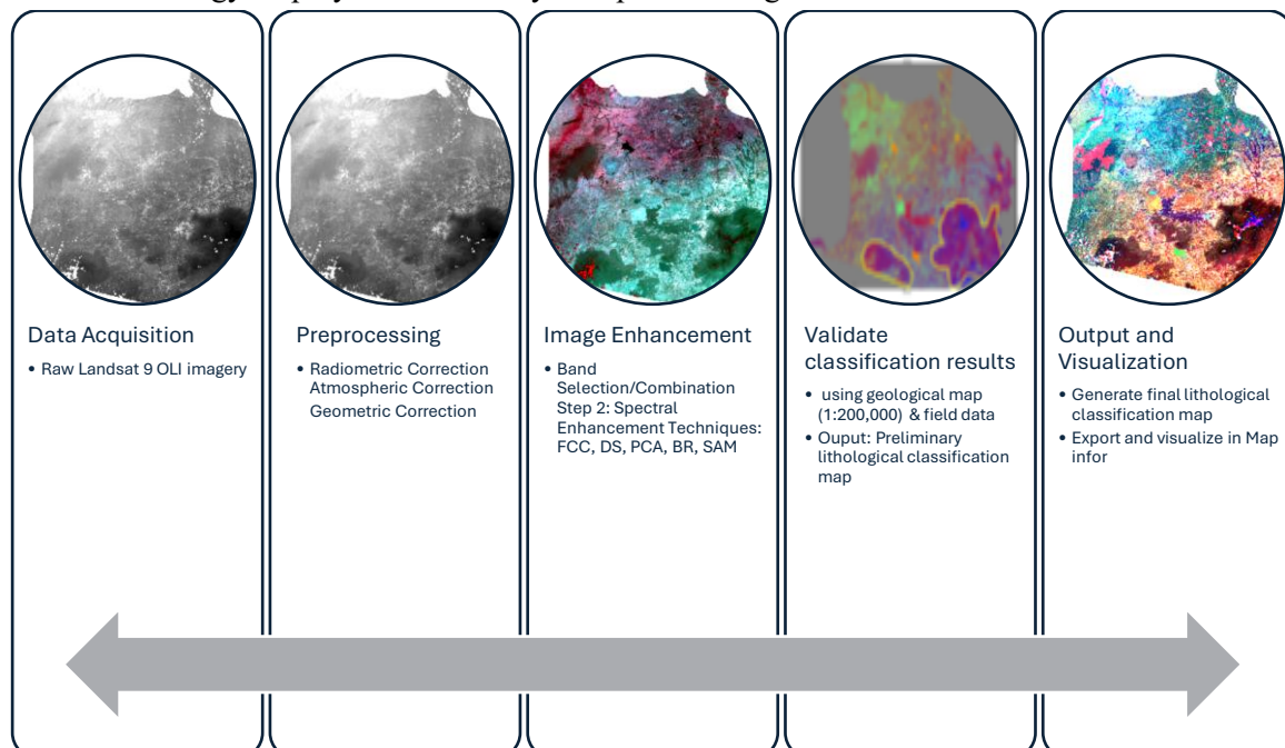
Fig. 2. Flowchart of the lithology classification process
