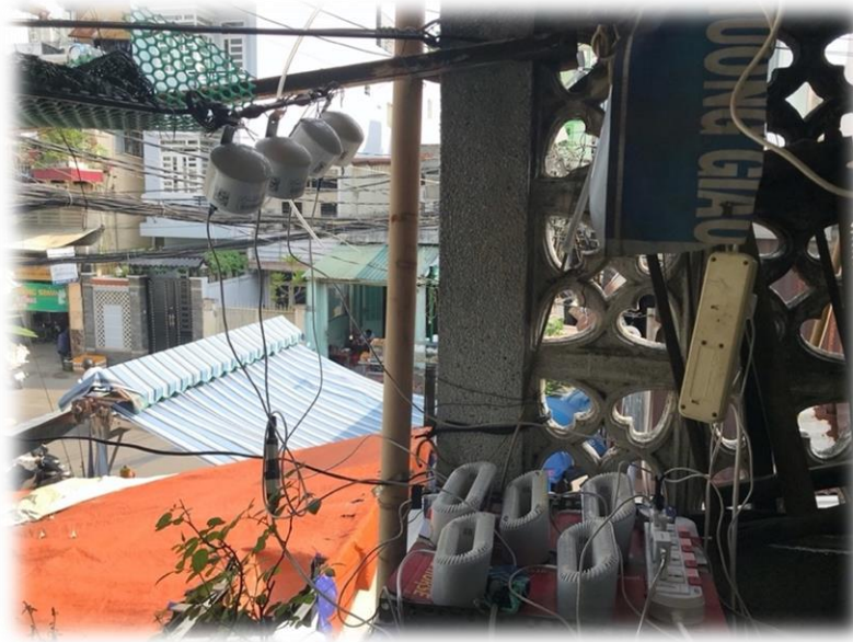
Fig. 2. (a) Indoor calibration and (b) outdoor calibration settings with all AirVisual and PurpleAir sensors in a household during 10 days in April 2021
